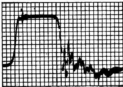
FIG. 4-5.—Voltage pulse at the grid of a 715B tube obtained from a regenerative driver using an 829 tube. Sweep speed: 10 div. per \mu sec; pulse amplitude: 1000 volts.
